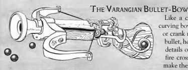
Like a crossbow, a bullet-bow consists of a stock, a curving bowstave and a bowstring drawn back by a lever or crank mechanism. The stock carries a barrel for the bullet, however, with a gap for the string. Certain other details of construction mean that bullet-bows cannot fire crossbow bolts or vice-versa. Built-in iron sights make the bullet-bow easy to use with minimal training,
